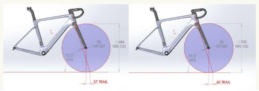
The secondary intended use for this bike outside of pure gravel racing is as an "Crossover" bike, with tires ranging from 28mm-35mm. The handling geometry was carefully selected to give "road like" trail values when used with a smaller outside diameter tire. The rear center length, higher hand position fit, and slacker HTA contribute to all day comfort. The bike has been registered with the UCI for use in road competition.
