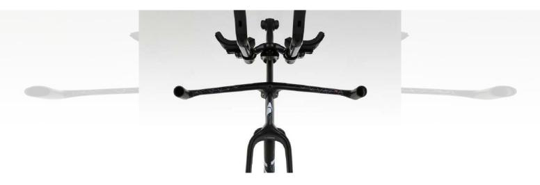
The HANZŌ uses never before applied airfoil sections for the full 16cm of length allowed by the alignment of the head tube and down tube boxes
